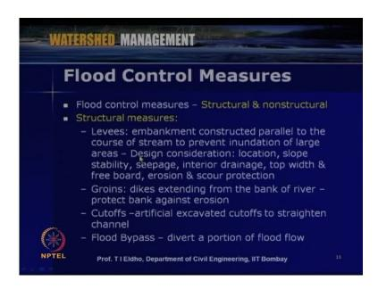
Levees are generally used to say, reduce the flooding problems wherever flood prone rivers.
