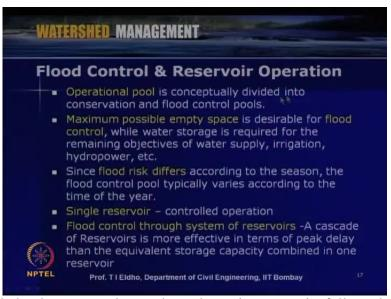
which controlled releases can be made and maximum static full pool. Actually, the difference between this minimum level and maximum static full pool is generally utilized for storage, and that can be effectively operated so that, if possibility of flooding is there, that can be reduced.
