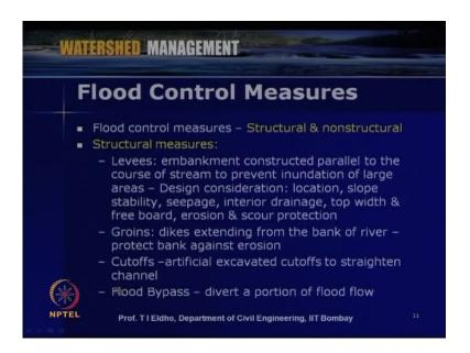
That kind of structure is called cut off, and then we can also have some structures like a flood bypass. This bypass means, wherever possibility of heavy flood in some regions, we can take the flow coming through certain other means like tunnels or the pipes or through some other channels, and then we can divert the flood flow.
