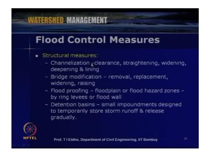
Then, some of the other structural measures include channelization. Channelization means, some of the activities, what we can do ,clear the channel, then we can straighten it, then we can widen it, then we can deepen it and also then the sides can be lined.
